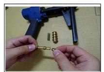
Separate valve unit (009), tube unit (008) and spring (004), Then replace valve's O-ring (512).
