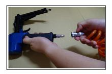
1. Disconnect the air supply from the tool.
