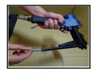
Insert D-rings into your tool following the instructions of loading the tool.
