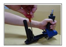
Separate screw (516) and magazine unit (024) with 3MM Hex, wrench key.
