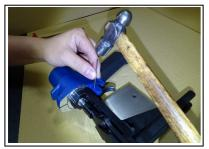
Separate spring pin (504) and trigger (003) with  $\phi$  2.8MM shaft and hammer.
