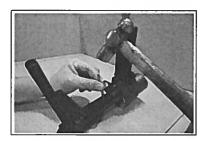
Take away spring pin (519) with  $\phi$  5mm shaft and hammer.
