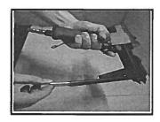
Insert D-rings into your tool following the instructions of loading the tool.
